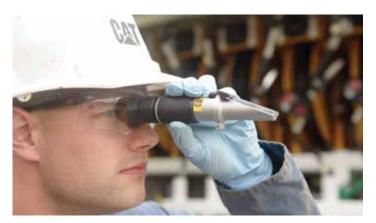
Too much or too little glycol will reduce the coolant's ability to provide protection to the cooling system. Heat transfer is affected by glycol concentration. Excessive levels of glycol will reduce heat transfer. Freezing Point and Boiling Point are calculated from Percent Glycol.
